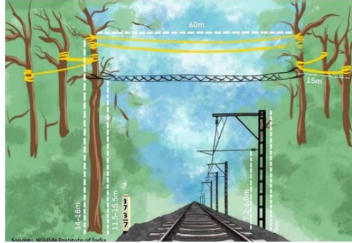
The canopy bridge designed by the Wildlife Institute of India for installation in a gibbon sanctuary in Assam, and, right, a Hoolock gibbon. SPECIAL ARRANGEMENT
