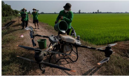
New ways of farming: A worker loads fertilizer into a tank attached to a large drone, preparing to spray it over the rice fields in the Long An province in southern Vietnam's Mekong Delta, on January 23. AP
