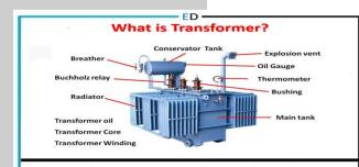
The transformer is a static device which is changes the voltage level and current level without changing the frequency. The transformer is used to increase or decrease the voltage and current level.
