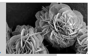
The carbon nanoflorets' high efficiency comes from three properties. First: the nanoflorets absorb three frequencies in sunlight infrared, visible light, and ultraviolet.
