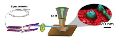
Synchrotron X-ray Scanning Tunneling Microscopy: Science-driven development of a next-generation instrumentation concept
