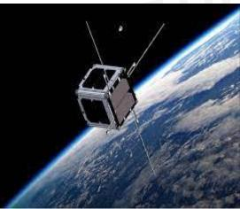
Starberry-Sense is ready for launch on the PS4-Orbital Platform by ISRO and can be used for CubeSats an\*/d other small satellite missions in the future.  The brain of the instrument is a single board Linux computer called Raspberry Pi.
