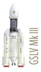
Height : 43.43 m Lift-off weight : 640 t Propulsion : Solid, Liquid & Cryogenic Payload mass : 4000 kg Orbit : Geosynchronous Transfer Orbit
